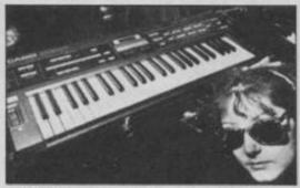
CASIO The Casio CZ series, CZ-101, CZ-1000 and CZ-5000, all use a digital sound generation technique called Phase Distortion Modulation, or PDM for short. The technology Casio uses to produce the sounds is a sort of hybrid of digital and analog circuits. They use digital technology to treat and modify a source sound to treat and modify a source sound wave in much the same way as
